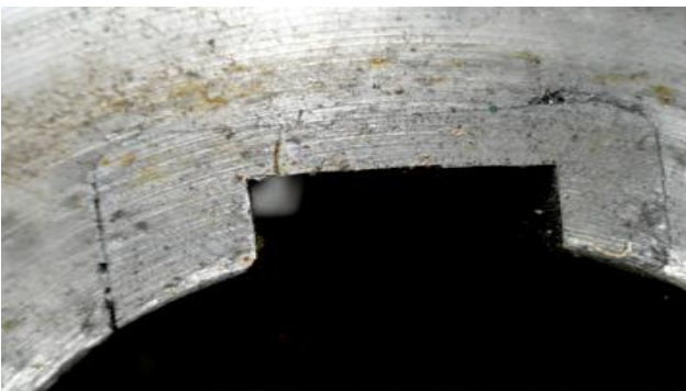
Figure 8 – Keyway in a wheel made of 300X28H2 cast iron with a steel insert made of Steel 3 after machining (Created by the authors)
