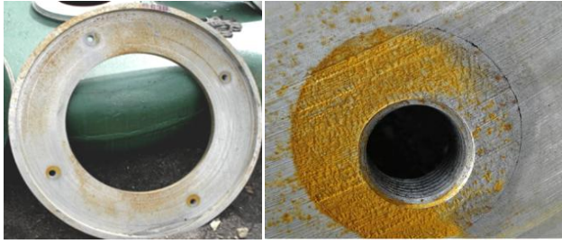
Figure 7 – Disc made of cast iron 300X28H2 with inserts made of steel Steel 3 after machining by cutting (Created by the authors)
